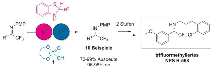
Chiral Phosphoric Acid Catalyzed Transfer Hydrogenation: Facile Synthetic Access to Highly Optically Active Trifluoromethylated Amines
